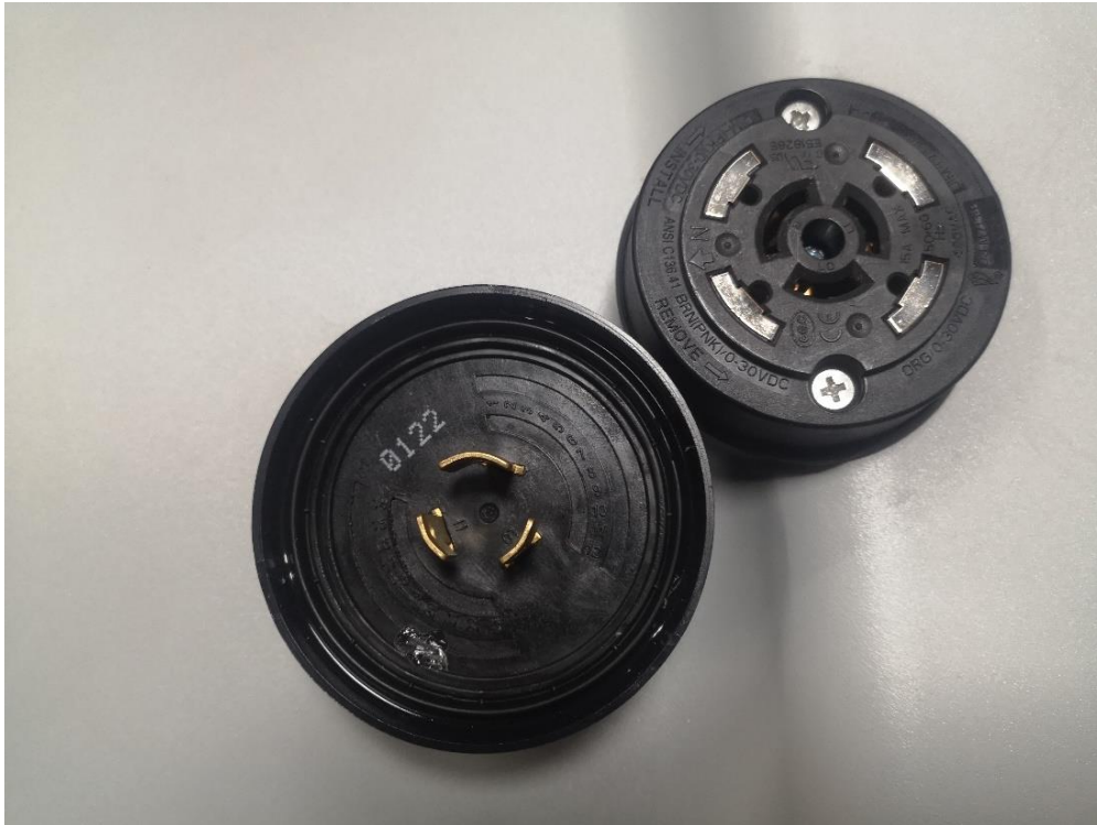
Picture 11.: NEMA socket with Shorting cap view
